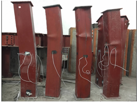
图 3 典型试件的破坏形态 Fig. 3 Failure modes of typical specimens
