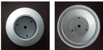
图 3 LED 散热体成形零件 Fig. 3 Forming part of the LED heat dissipation body
